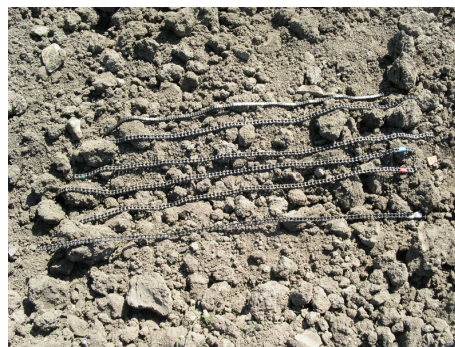
Figure 3. Chain set. Field measurements. Soil tilled with chisel.
